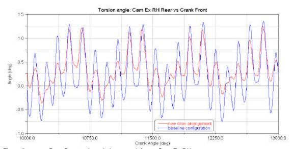
Figure 5. Rear Cam torsion relative to crank front – Cam Ex RH
