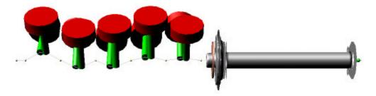
Both the crankshaft and dyno driveshaft were modelled as flex bodies. Previous analyses had shown that crankshaft torsion is sensitive to model detail within the drive arrangement. This model was created before the age of A/Engine Cranktrain, so the valvetrain interface had to be modified to create cranktrain subsystems. Faster run times may now be possible using the FEV beam crank.
