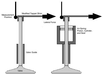
Figure 2. Test configurations for verification of flexible valve model
