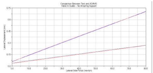
Figure 3. Comparison of valve lateral stiffness with test
