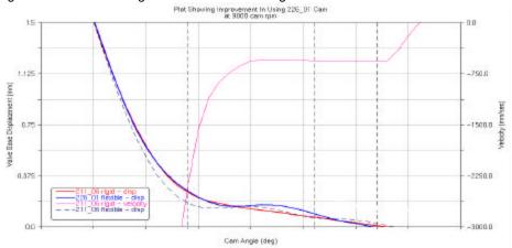
Figure 10. Showing how a cam profile change can improve valve control
