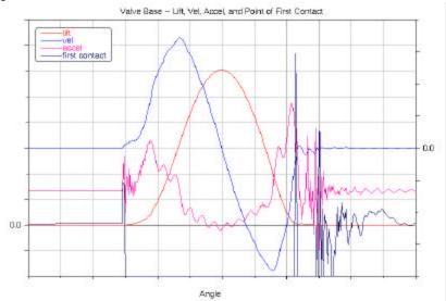
Figure 7. Lift, velocity, acceleration and seat contact force at 9000 cam rpm
