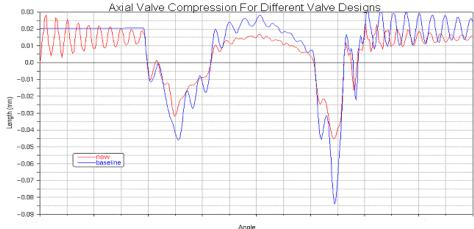
Figure 8. Axial valve deformation – showing improvement in new valve design
