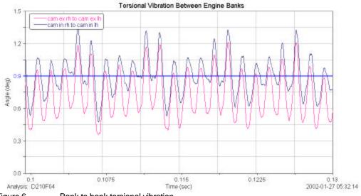
Figure 6. Bank to bank torsional vibration
