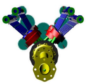
All cams were constrained so that all the valves were on their seats at the start of the analysis. Imposed motions then moved the cams into their required position within the first camshaft revolution (thanks to Christoph for this one). This was required as ADAMS was having difficulty finding static equilibrium when some of the valves were at maximum lift (>15mm worth of movement).
