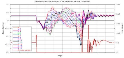
Figure 9. Showing axial d eformation at edges of valve base
