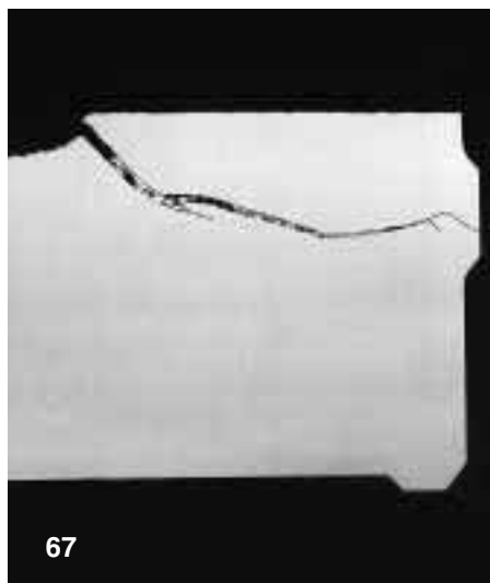
Fig 67 Cross section through the roller depicted in fig 66, showing the way in which the fatigue crack extends beneath the surface. The fully developed flaking originated in the same manner
