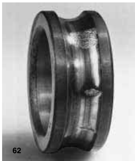
Fig 62 Various stages of flaking in the inner ring of a deep groove ball bearing. The ring has been mounted with interference fit on the shaft and blows have been directed against the outer ring, causing the mounting force to pass through the balls, which have produced the indentations
