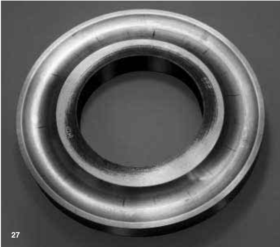
Fig 27 Washer of a thrust ball bearing subjected to overloading while not running. The indentations are narrow and radially aligned, not sphered as in radial ball bearings
