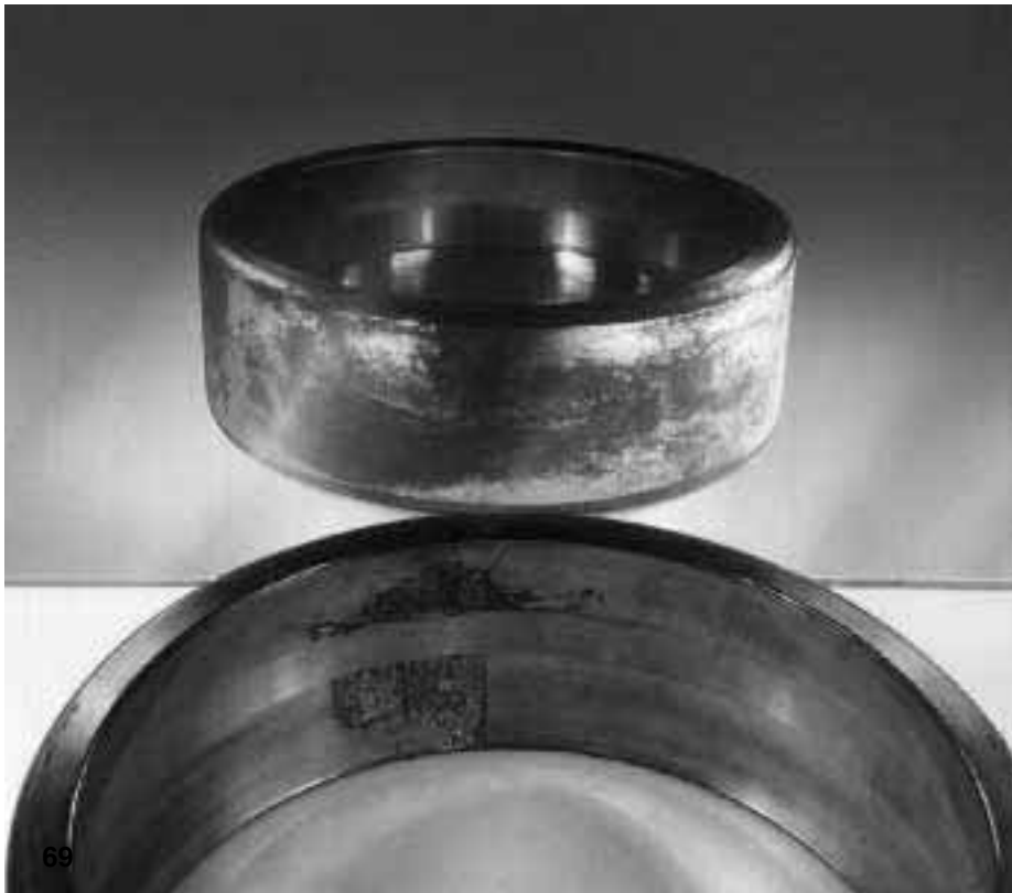
Fig 69 Flaking in the raceways of the outer ring of a spherical roller bearing. Corresponding area of advanced fretting corrosion on the outside surface (for this photograph the ring has been placed in front of a mirror). Development of the corrosion has been accompanied by an increase in volume that has led to deformation of the bearing ring and localised overloading. The results have been premature fatigue and flaking
