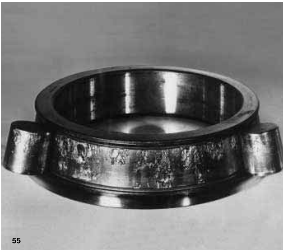
Fig 55 Flaked cone and rollers of taper roller bearing. Heavy loading and inadequate lubrication are the causes of this damage
