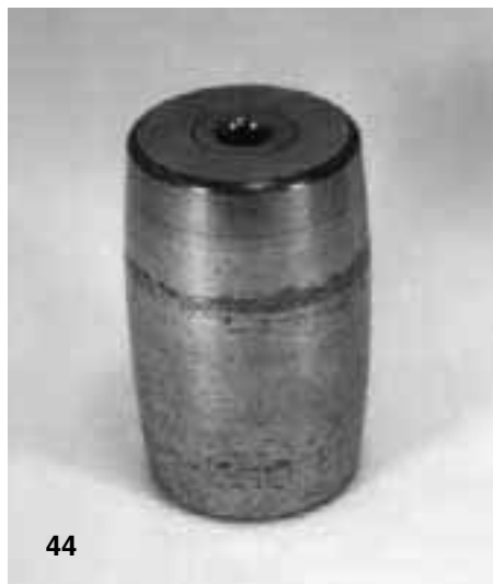
Fig 44 Surface distress in the form of a band encircling a roller from a spherical roller bearing
