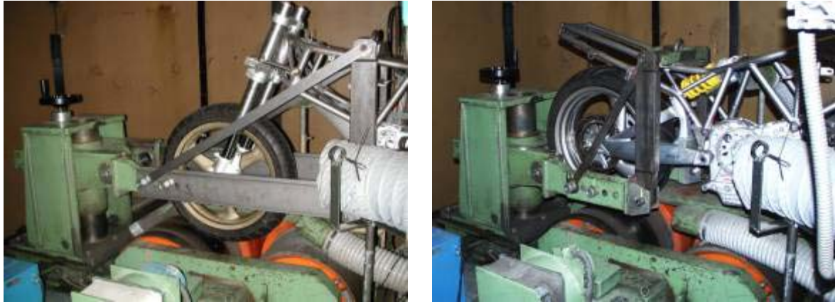
Fig. 8: Fatigue test bed for the front and rear.
