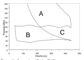
Figure 10. Conventional Engine PV Diagram
