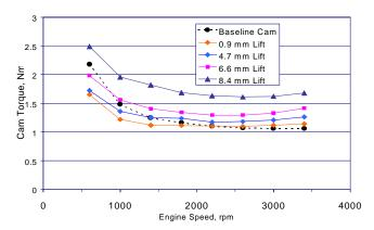
Figure 8. VVA Mechanism Torque
