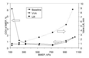
Figure 18. COV of IMEP v. BMEP at 2000 rpm
