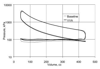
Figure 11. Pressure v. Volume: 2000 rpm / 800 kPa
