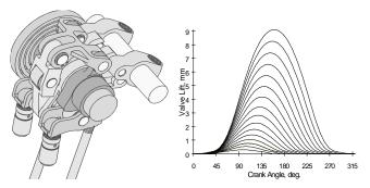
Figure 2. VVA Mechanism Configuration and Lift Curves
