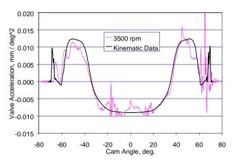
Figure 7. VVA Valve Acceleration at 3500 rpm / 8.9 mm lift
