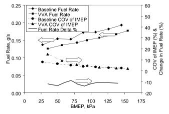
Figure 14. Idle Performance at 750 rpm
