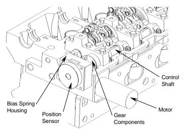
Figure 4. Actuator installed in cylinder head
