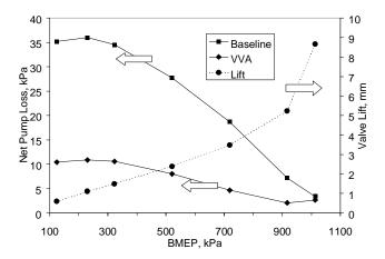
Figure 17. Net Pump Loss v. BMEP at 2000 rpm
