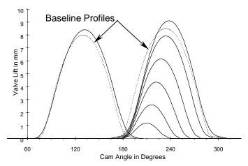
Figure 9. VVA Cam Timing and Baseline Lift Curves
