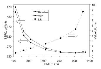
Figure 15. BSFC v. BMEP at 2000 rpm
