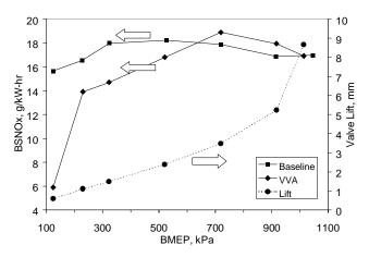
Figure 20. BSNO<sub>x</sub> v. BMEP at 2000 rpm
