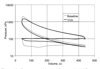
Figure 12. Pressure v. Volume: 2000 rpm / 300 kPa NMEP
