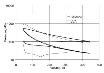
Figure 13. Pressure v. Volume: 2000 rpm / 100 kPa NMEP
