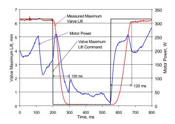
Figure 5. Control System Step Response
