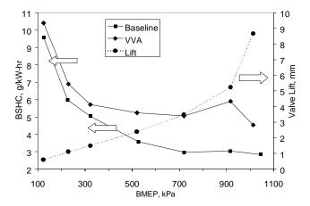
Figure 19. BSHC v. BMEP at 2000 rpm
