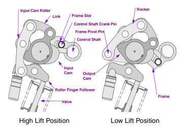
Figure 1. Roller Finger Follower VVA Mechanism
