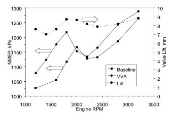
Figure 21. Full Load NMEP v. Engine Speed
