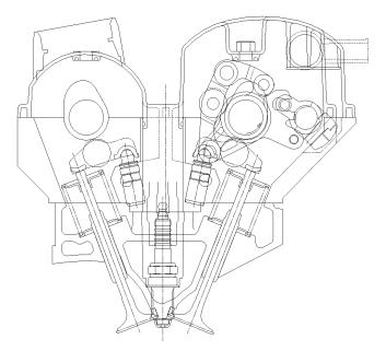
Figure 3. Dynamometer Engine Cross-section
