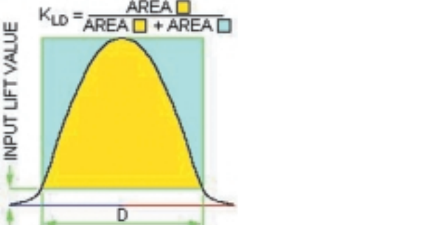
Figure 5. The lift duration envelope is calculated at every iteration of the design.
