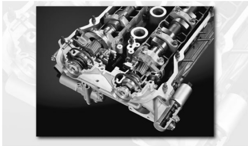
Figure 7. Double VANOS variable camshaft control on BMW 6-cylinder engines
