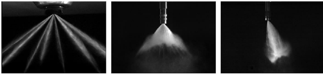
Figure B.1: Typical spray patterns of different atomization concepts, (left) multi-hole, (middle) outward opening, (right) inward opening swirl type, [179].
