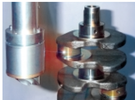
Laser structuring of a crankshaft
