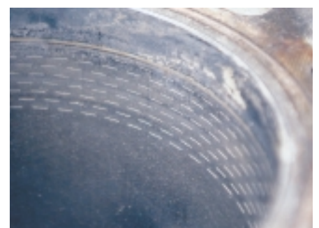
Cylinder wall after 160,000 km
