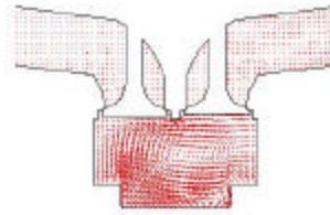
Fig.18 Fluid flow pattern in xz plane, y=0 , at 300 deg. ATDC (SA=54%)
