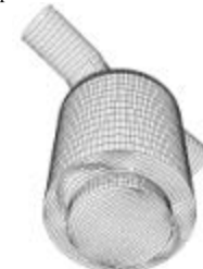
Fig.11 Perspective plot of the cylindrical combustion chamber (SA=54%) with valves
