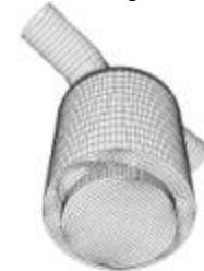
Fig.10. Perspective plot of the cylindrical combustion chamber (SA=44%) with valves
