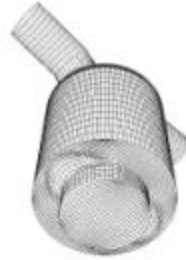
Fig.12 Perspective plot of the cylindrical combustion chamber (SA=63%) with valves
