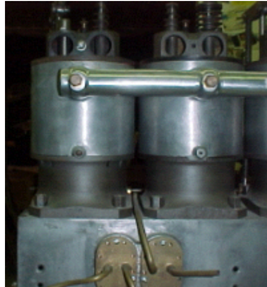
Figure 2 – Engine Details Showing Auxiliary Ports And Cooling Jackets
