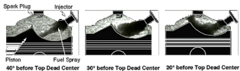
Figure 1: GDI Fuel Injection Pattern (during compression stroke)
