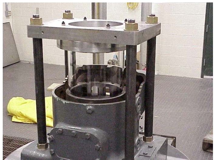
Figure 3 Picture of 36 cm bore optical engine.
