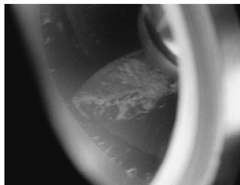
(c) Cavitation on impeller at 95°C deaerated to 33 ppb, NPSH_{av} = 8.06 m, rated flow
