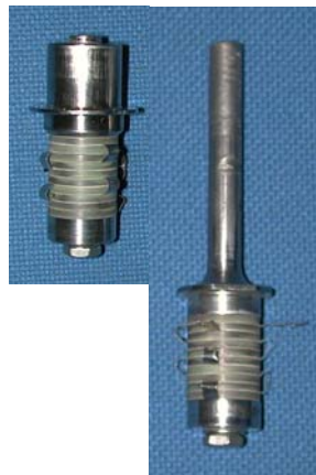
Figure 7. Photograph of the folded horn (16 kHz) and a comparison of a straight horn with approximately the same frequency(20 kHz).
