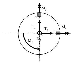
Figure 8. Load on a pin section: bending moments  $(M_x, M_y)$ , torque moment  $(M_z)$ , normal force  $(N_z)$ , shear forces  $(T_x, T_y)$
