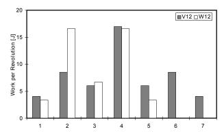
Figure 14. Comparison between friction losses in each crankshaft bearing of a W12 and V12, at 18000 rpm.
