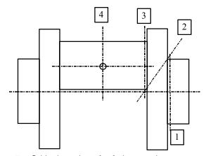
Figure 7. Critical sections for fatigue resistance
