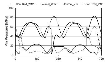
Figure 9. Pressure on the crankpin and journal against crank angle
