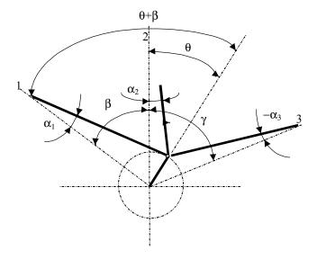
Figure 6. Sketch of the crank with the connecting rods
