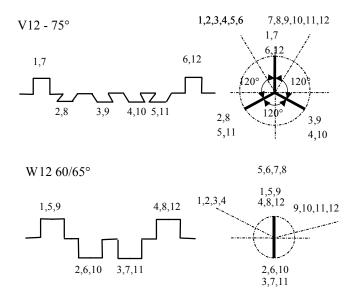
Figure 10. Sketch of the V12 and W12 crankshaft
