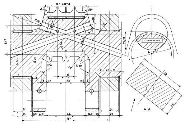
Figure 3. Working drawing of one V12 crank
