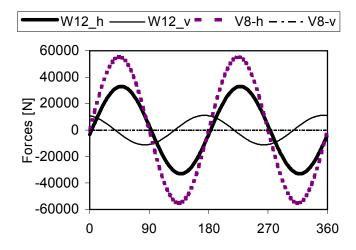
Figure 12. Unbalanced crankshaft forces.
