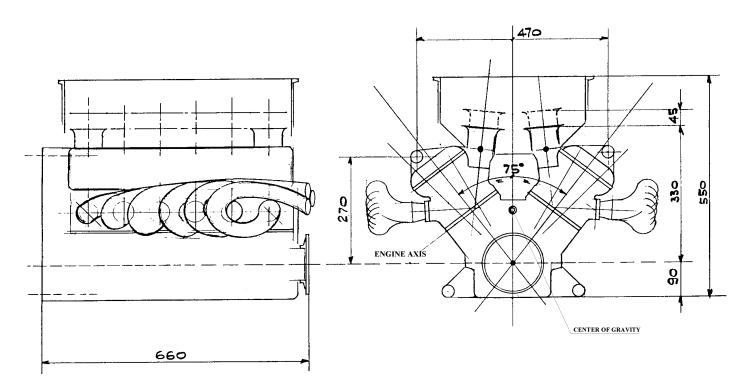
Figure 2. Lay-out of a traditional V12 engine. The engine is connected to the cockpit by 4 points.
