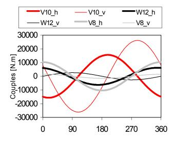
Figure 13. Unbalanced couples regarding crankshaft's left end (cockpit side)
