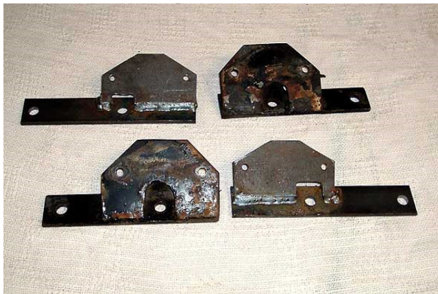
Modified motor mounts (shown upper-left and lower-right) put the engine about a half inch lower than "normal".
