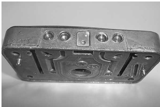
Metering Block (note the dimple that has to be drilled out for screw/rivet)
