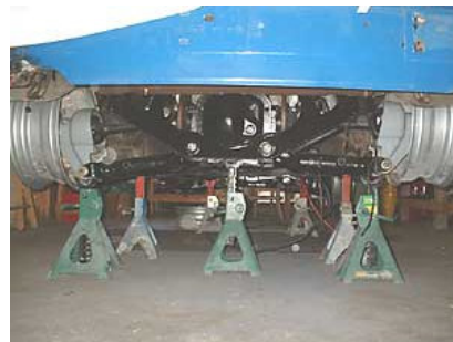
Jaguar IRS: rebuilt, narrowed & installed in MGB
