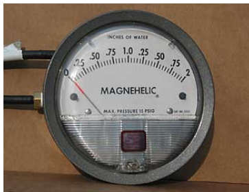
Magnehelic gauges are 4.5" in diameter and have two sets of 1/8" NPT ports.
