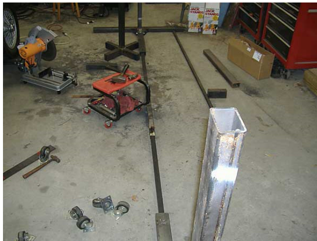
Stand base showing bolt on leg.
