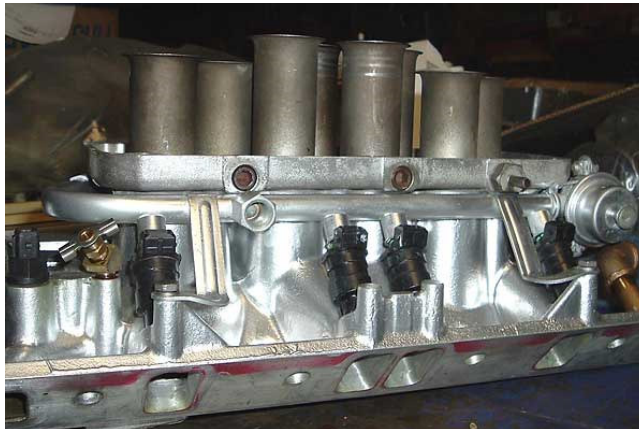
The fuel rail can be lowered slightly by tweaking its mounting feet.
