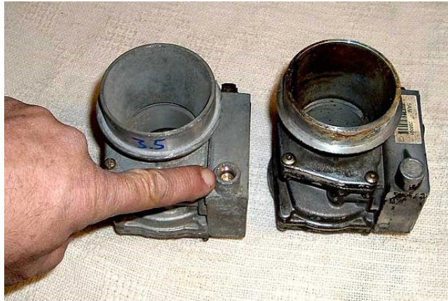
Mass Air Flow (MAF) sensor. (At left, a "tamper proof" plug has been removed to reveal the idle speed adjustment screw.)
