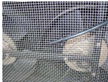
1/8" I.D. crush-resistant PVC hose is routed from the gauge to areas of interest.
