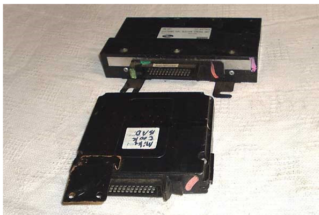
Two generations of Lucas ECU. (Foreground: 14CU or 14CUX. Behind it: 13CU.)
