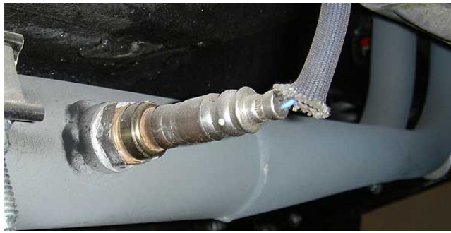
Typical installation of an oxygen sensor for an aftermarket air/fuel meter.
