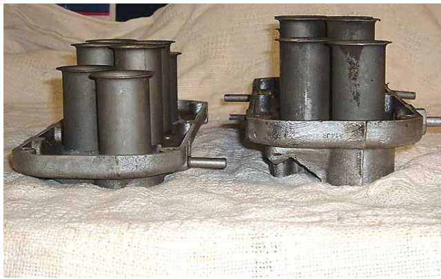
Glen mills 0.800" off the bottom of the Plenum Base to add hood clearance.
