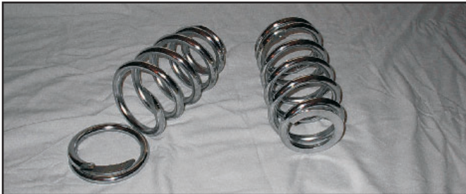
Photo 2: New coil over springs before and after cutting.
