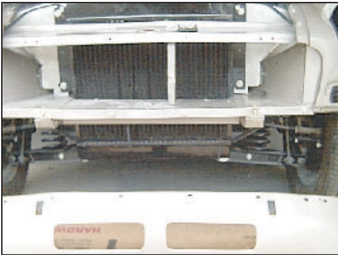
Heavy duty radiator fitted. Air holes put in front valance to increase air flow.
