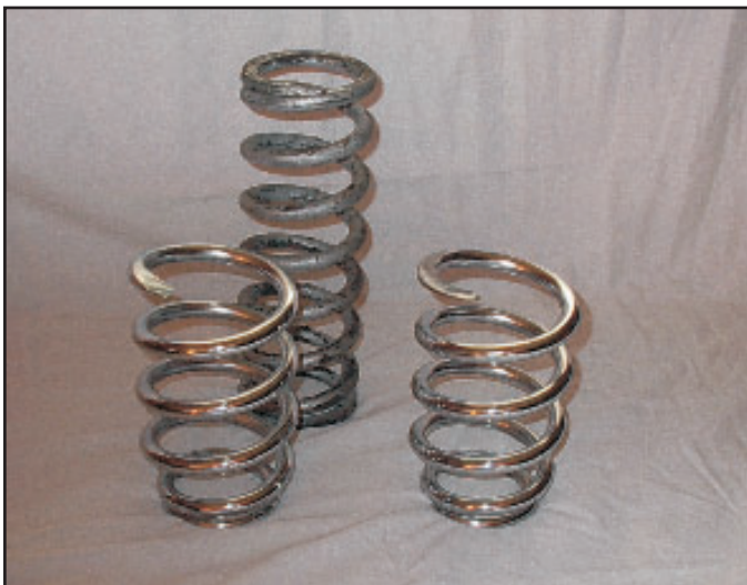
Photo 3: Stock springs compared to the cut-down coil overs.
