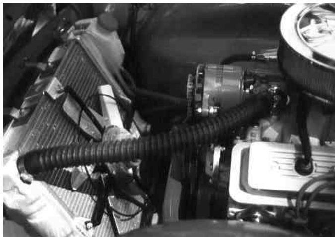
Chevy 350 with a Griffin aluminum radiator & electric fan. No cooling problems at all with this setup
