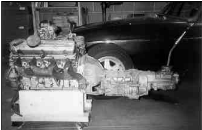
Originally installed Olds 2-bbl engine with Borg-Warner T-50 5-speed transmission. Note Buick 300 exhaust manifold.
