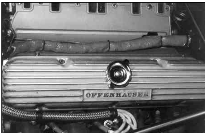
Engine wiring is run through a heat resistant fiberglass/silicone tubing and routed under intake manifold.
