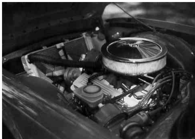
330HP Chevy 350, Edelbrock Performer intake manifold, Holley 600CFM center pivot carburetor, BW T5 transmission
