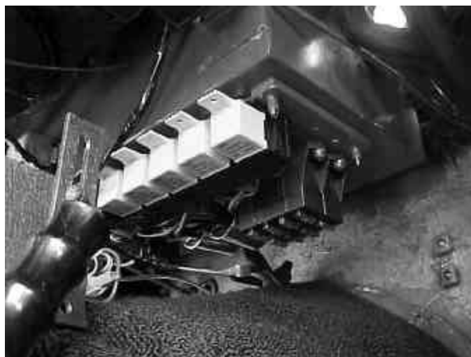
Power Block as installed in a TR3. In this car, the best location for the block was under the battery box, behind the dash.
