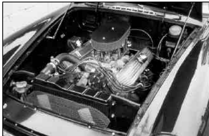
Olds 215 with dual Rochester 2-bbl carbs, Edelbrock intake, and Offenhauser cast aluminum valve covers.
