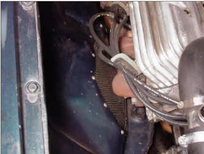
Photo 3 Duct and grill installed in inner fender panel adjacent to exhaust header.
