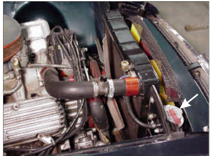
Photo 1 Cooling system with tee in top hose, stock MG fans and fabricated overflow tank (arrow)
