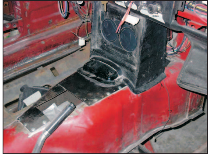
Trans tunnel mods. Note the AC ducts in the dash support
