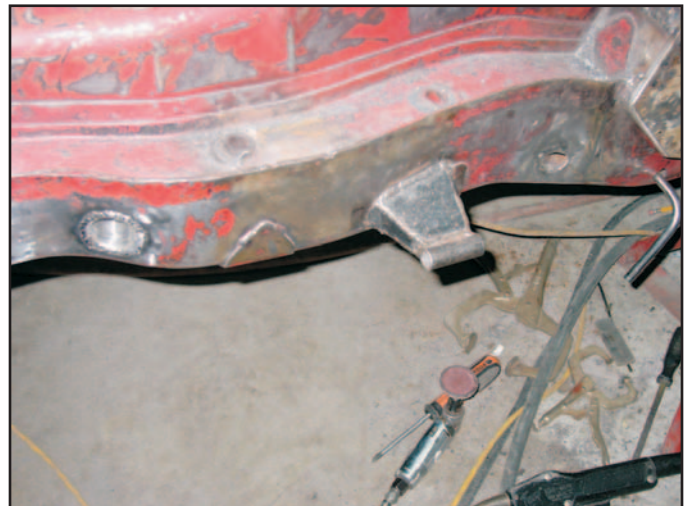
Motor mount, outlet for hidden wiring, and fuel line outlet
