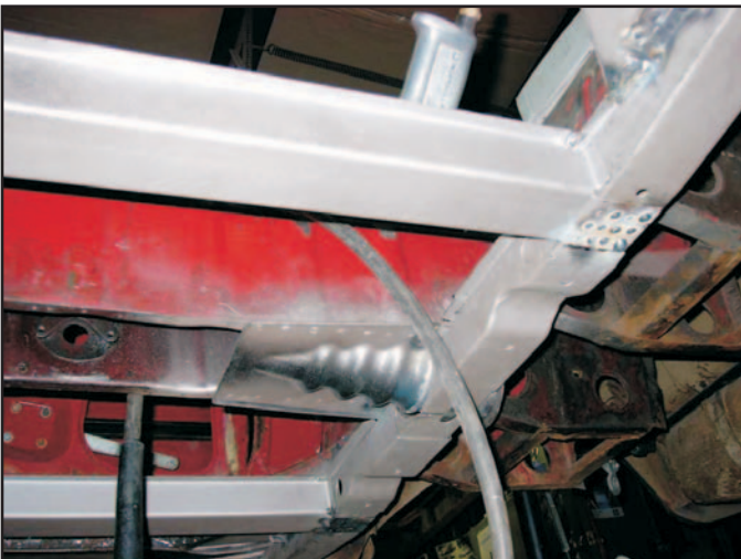
Additional U-channel frame stiffeners
