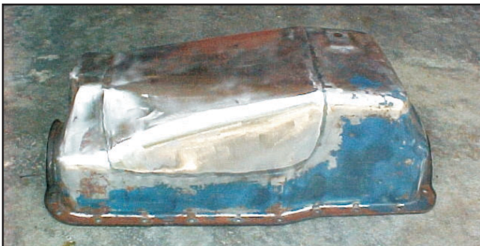
Photo 5: A little cleanup, a little paint, and Voila! a rear sump oil pan on the cheap.
