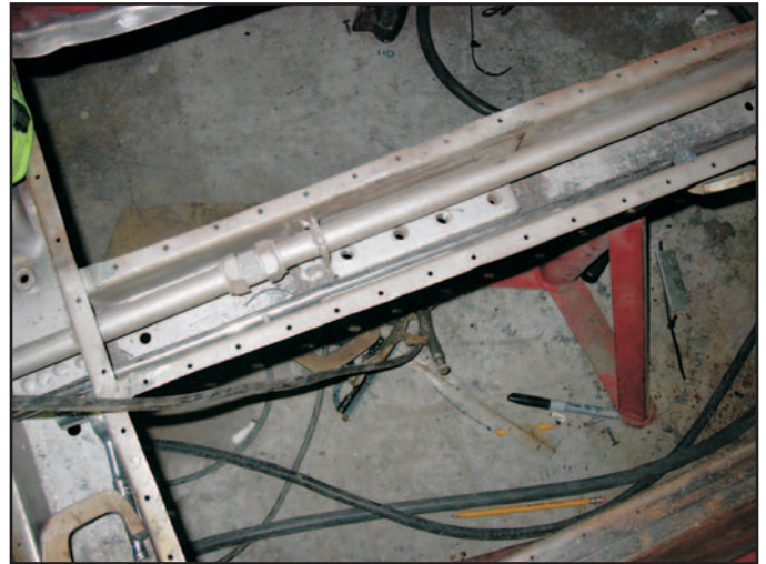
Wiring to the rear is routed through this conduit! Neat idea!
