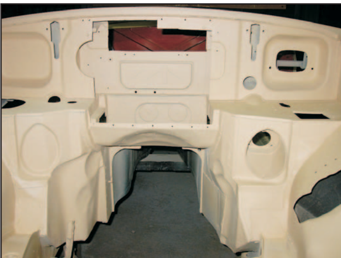
Completed firewall mods, including cutout for A/C unit
