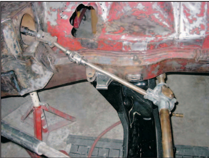
Completed engine mount and brackets for the steady bars
