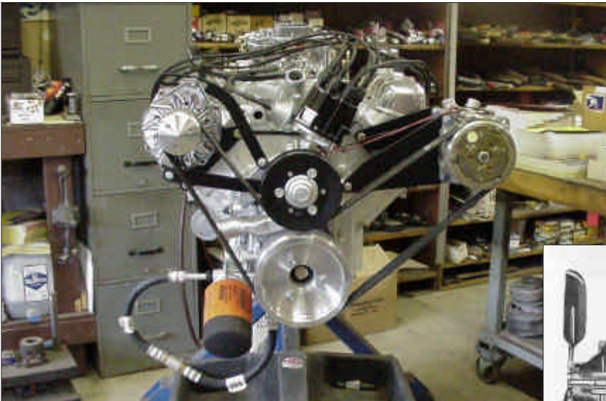
Dave Michel's 348 cid Buick 300/350 hybrid engine
