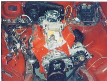
CHEVROLET 60-DEGREE V6 MGB INSTALLATION KIT
