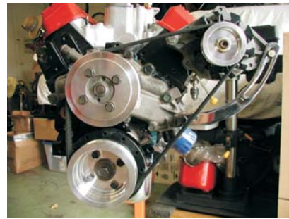
THREE PIECE PULLEY SET FOR CRANK, WATER PUMP AND ALTERNATOR
