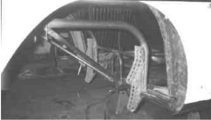
Plenty of adjustment available for the 4-link bars
