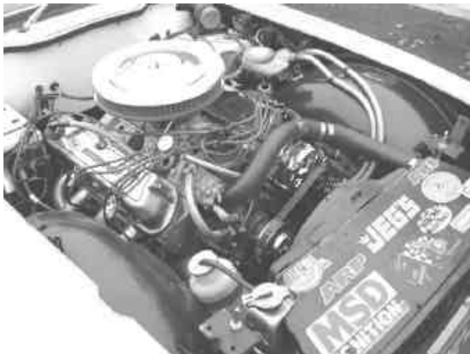
450+ HP! Note the full radiator shrouding in front and in back of the radiator
