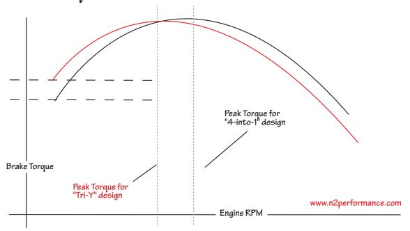
Note: Although somewhat exaggerated, these two torque curves depict basic differences in characteristics between a typical "Tri-Y" design and a "4-into-1" layout, as applied to a V8 engine. Depending upon primary pipe sizes, the two may exhibit different peak rpm points, but the ability of a "Tri-Y" to increase low rpm torque is typical, as compared to the "4-into-1" design.
