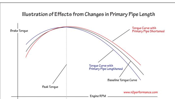
Note: Since peak torque rpm (as affected by the exhaust system) is largely determined by primary pipe area, lengthening and shortening primary pipes tends to "rock" the baseline torque curve about this point.
