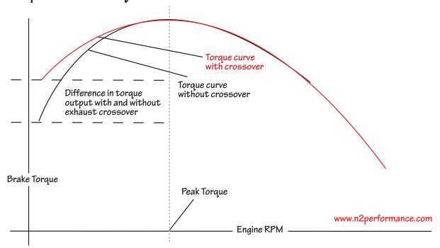
Note: In much the same fashion that a header collector "works" below and up to peak torque rpm, crossover pipes provide gains in a similar range or engine speed. If an engine is carbureted, the addition of a crossover typically requires a change to enrichment.
