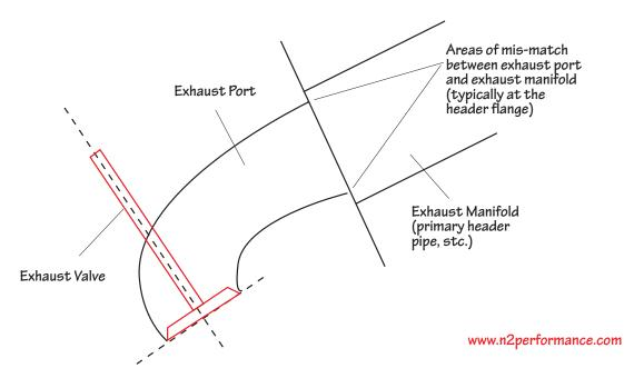
Note: Some measure of reversion containment can be accomplished by a physical mis-match between exhaust port and exhaust manifold (typically a header primary pipe) by allowing pipe l.d. to exceed port l.d. This mis-match is often accomplished at the exhaust header flange-to-head interface.
