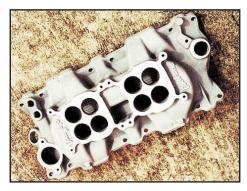
To simplify carburetor linkage assemblies while still providing additional carburetor throat area, in-line 4-bbl carburetors became a popular performance path. Such systems were also adopted as OEM options adding performance benefits beyond that obtainable with single 4V carburetion systems. Manifold design was limited to incorporating the 180-degree firing order pattern, as pioneered by Vic Edlebrock, Sr. in the 1940s.
