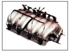
This so-called "folded hands" design is used on current Chevrolet LS1 (and LS1-type) engines. Fuel injector nozzle location is highly critical and formed the basis for much of the manifold (and cylinder head) design. Runners in this manifold are specifically intended as "extensions" of the cylinder head inlet ports. Long runners add to low- and mid-rpm torque output.
