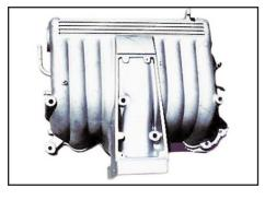
Stock FoMoCo manifold for 5.0L Ford V8 incorporates long individual runners, terminating in an intake manifold base providing paths to each cylinder head inlet port. "Plenum" function is provided by long flow path (volume) leading from throttle body mounting flange to entry of "air box" (additional plenum) to which all runners are connected.
