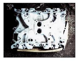
Due to low profile hood lines, some OEM intake manifolds were of single-plane design. Adding to the complexity of latemodel intakes is the requirement for internally plumbed exhaust gas re-circulation (EGR) passages and exhaust crossover paths for additional carburetor (or TBI) heat. Manifolds of this type frequently compromise cylinder-to-cylinder mixture distribution in favor of packaging requirements.
