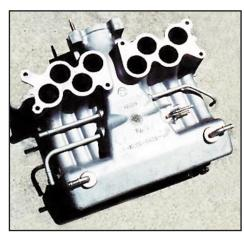
Belly-side of Ford 5.0L manifold reveals shape of "air box" and throttle body path, tapering from TB flange into the box. Runner exit ports are staggered to allow alignment of cylinder head inlet ports; including bank-to-bank port stagger due to cylinder offset (bank-to-bank).
