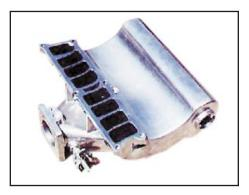
Belly-side of Holley "SysteMAX" design reveals enlarged port runner cross section areas and aligned (although somewhat spread) inlet ports-to-manifold arrangement. Bank-to-bank off-set is compensated by spreading ports in manifold base, causing a measure of inclination of end ports to enable proper alignment between upper and lower parts of the manifold.
