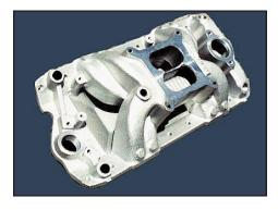
To further aid improved air/fuel mixture quality and condition, some inlet manifold incorporate gap" feature. "air This approach provides air circulation between manifold runners and the valve lifter galley cover, typically subjected to elevated oil temperature from underside exposure to the lifter galley. Early use of this technique was limited to racing manifolds, now incorporated in high performance street designs like this Edelbrock version.
