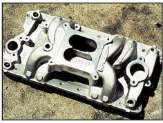
Today, intake manifold design sophistication relies less on multiple carburetors but more to the improvement of both airflow quantity and quality. Large 4V carburetors provide ample throat area, so refinement of manifold plenum chambers and runners enable a wide range of rpm in which power gains are obtainable.
